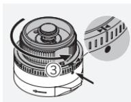
Turn the turret 35 clicks counter-clockwise and align the >|< marking on the top of the scale with the index point. Then
