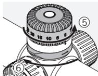
Now you can choose the settings you want on the turret. Rotate the locking mechanism one quarter turn clockwise to lock it.
