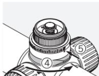
Open the locking mechanism on the turret. Turn the marking on the turret to zero if it has moved to another position.
