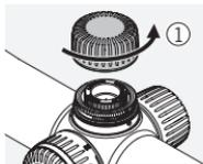
Remove the screw-on cap from the top turret of the scope.
