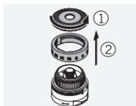
Unscrew the knurled ring from the turret. Remove the knurled ring and the graduated ring (or the marking rings).
