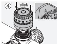
Install the turret to the scope until you hear a click. Note the zero position while doing this.
