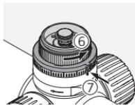
Put the marking rings on the turret on the basis of the information in the ballistic program and align them with the index point.
