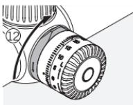
Rotate the locking mechanism one quarter turn clockwise to lock it.
